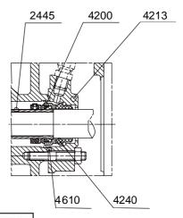
With a mechanical seal, the maximum temperature is limited to 80 °C (176 °F) whatever the internal construction of the pump is (Cast iron or Bronze).
